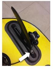
Turn the vessel around. To place the motor fins correctly, make sure that the motors are on the outside. Slide the fins in their place and fasten the bolt to secure that the motor no longer comes loose. Put the two cables of the motors through the closest hole of the vessel and turn the boat around again.
