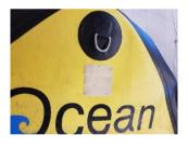
On the bow of the calypso inflatable boat, a Velcro patch is provided to place the compass and keep it in place.
