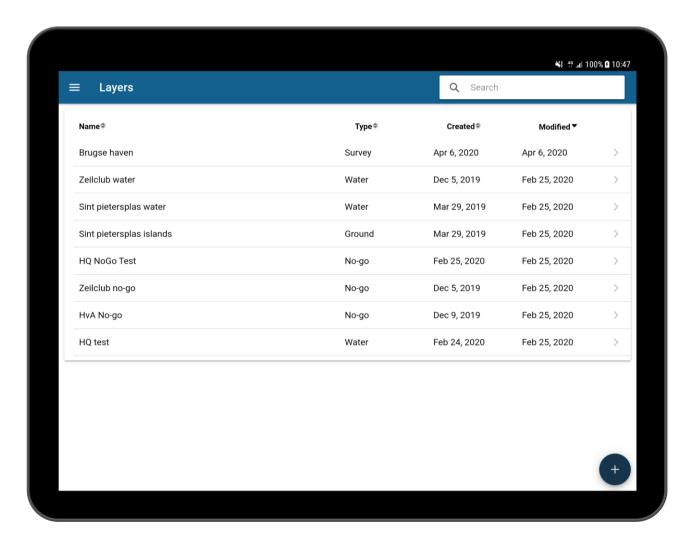
The list of layers can be accessed by going to the AYB menu – Layers. These layers will be used to calculate waypoints for the tasks. To successfully do that create a water layer where it is safe to sail and other layers (Ground, Pier, Bridge, No-Go) where it is not safe to sail. The path planner will take all the layers into account and try to calculate a valid route. Survey layers are passive layers and are only to mark the survey area (dashed border line).
