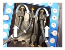
Before connecting the motor cables, make sure the AYB unit is not switched on. Remove the dummy connectors from the left and right connector by turning them to the left and pulling it out. Now connect the motors to each side of the connector compartment by plugging it in and turning the fastener to the right. Make sure the pins from the connector line up to each other. If the vessel is not turning the right way in the water, it is possible that the connectors are swapped.
