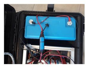
Before installing the battery, check if the emergency button is pushed in. Open the box by lifting every fastener. Place the battery in the provided compartment next to the drive unit. Next connect the cables of the AYB box to the battery. If everything is installed, close the box and secure every fastener of the case again. Make sure no cables are stuck between the box and the lid.
