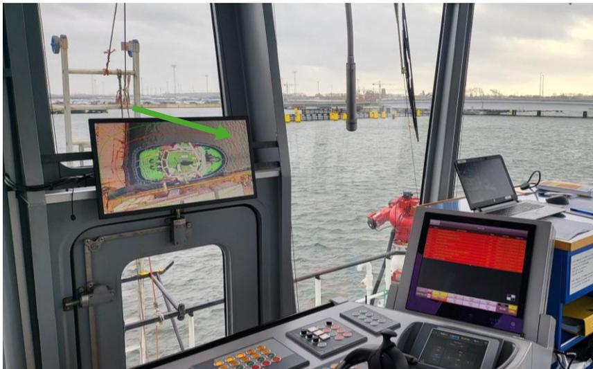
Figure 18: Installed monitor with dimmer on the left
