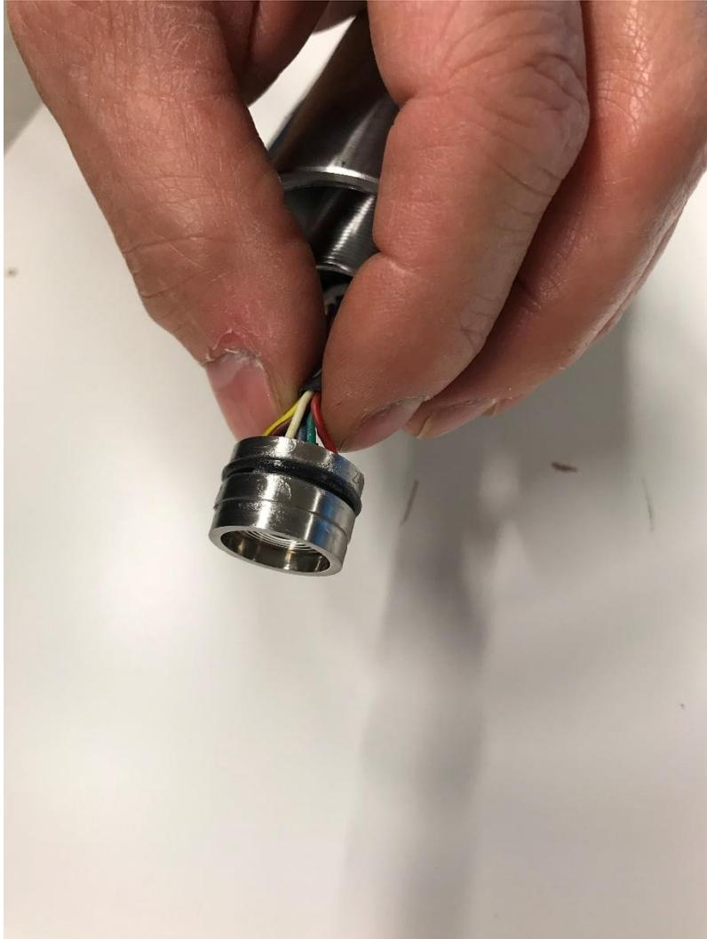
Put a little Vaseline on the outside of the sensor (seal). Then push the wires to the inside of the GraviProbe and push the sensor in place.
