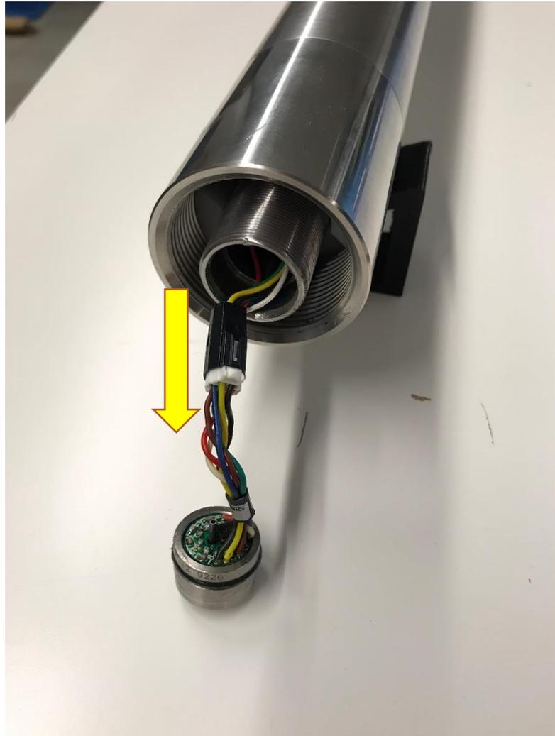
Disconnect the damaged sensor and reconnect a new sensor.
