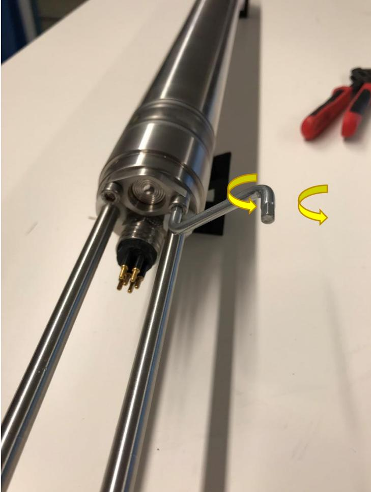
Take the included umbraco key and loosen the two screws.
