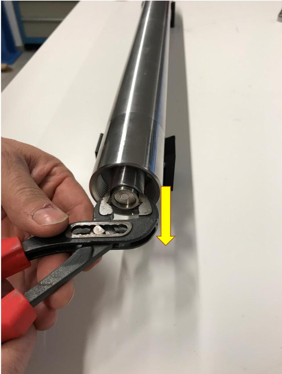
Take the pipe wrench and put it on the outside of the sensor, then carefully pull out the sensor by wiggling a bit.
